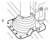
Fasten the muff on to the MetecnoSpan® external profiled sheet (distance between screws equal to 50mm); then install the collar
