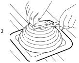
Adapt the muff to the pipe. Cut the opening so as to be at least 25mm smaller than the pipe diameter in order to overlap the pipe at least 20mm
