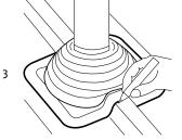
Fold up the muff on the pipe, Eventually using white liquor (soap) adapt the muff to roof profile and Mark out the contour
