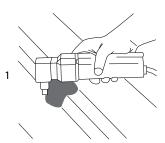
Prearrange the hole for the pipe. Muffs must always be placed on top of the profiled sheet top in order to permit the water flow
