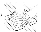
Place the muff by pressing it to the roof surface
