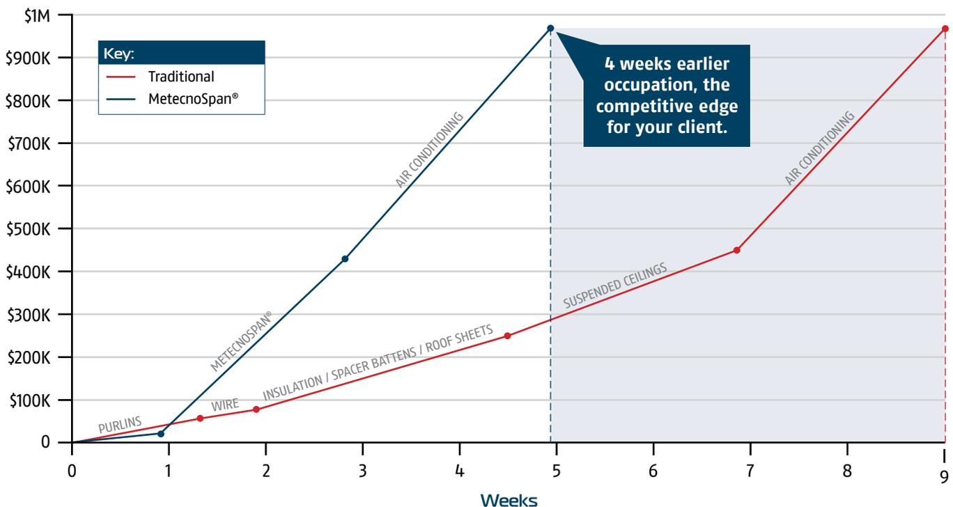
Typical construction segment timeline – 3,000m<sup>2</sup> air conditioned showroom.
