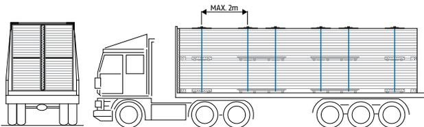
Fig. 5. Positioning of Panel Packs and Cargo Strap.
