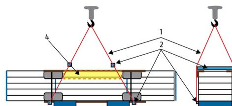
Fig. 7. Unloading of Panels of < 8.0m: 1. Lifting Sling; 2. Sling Separator (Timber/Channels).
